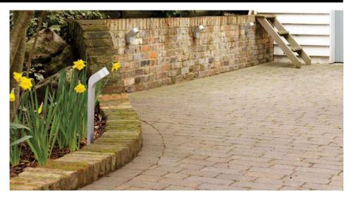
The **Soprano** guide light produces a low level light source to provide illumination of paths, driveways and walls. A compact fluorescent lamp is used instead of standard incandescent lamps to increase energy efficiency.
