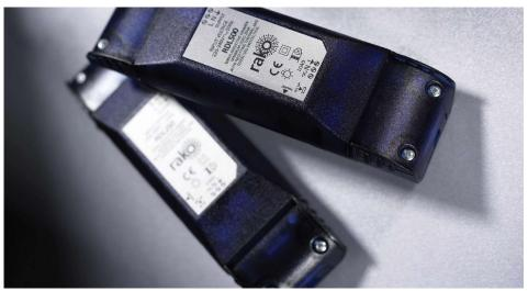
The **RAKO Constant Current Dimming Driver** is a wireless three channel (RGB) 36W constant current dimming LED driver. Up to 12 LED can be connected in series to a maximum of 12W on each channel. The maximum current settings are selectable from 350mA, 500mA, 600mA and 700mA. The unit requires up to 48V 36W DC power supply (RAKO RAPSU48-36).
