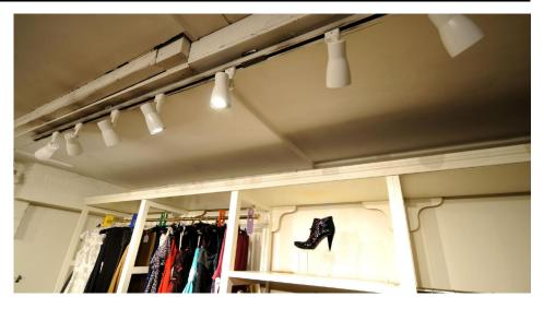
The **Long Nose PAR16 Spotlight** is a surface mounted spotlight used for general lighting. It has a longer body than standard GU10 spotlights, meaning that elongated bulbs such as LED retrofit lamps can be used without the light source protruding.
