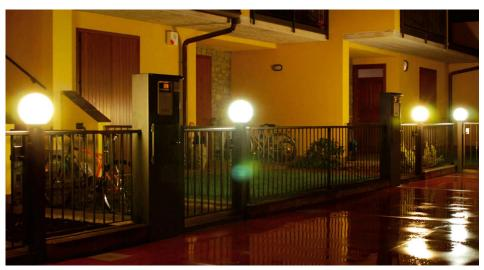
The **Globe** fitting is made from moulded and blown PMMA acrylic and comes in four different finishes: clear, smoked (a transparent brown finish), opal (opaque white) and metallic (half clear and half mirrored to reflect light downwards and reduce light pollution). It can be used on its own or combined with a variety of accessories to achieve the following different setups:
