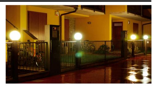
The **Globe** fitting is made from moulded and blown PMMA acrylic and comes in four different finishes: clear, smoked (a transparent brown finish), opal (opaque white) and metallic (half clear and half mirrored to reflect light downwards and reduce light pollution). It can be used on its own or combined with a variety of accessories to achieve the following different setups:
