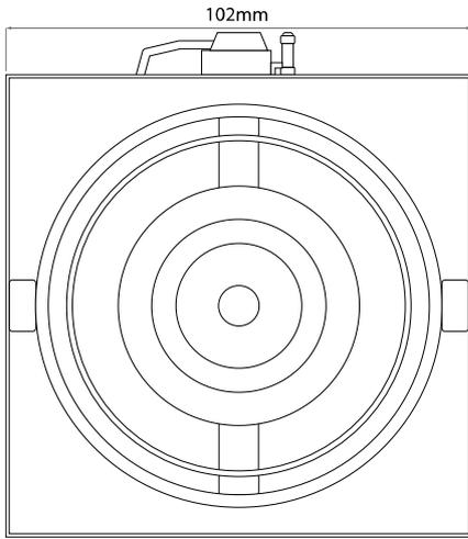
Section drawing for FRT100 Frame 15mm
