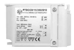
Dimmable output current 0/350mA. Equipped with push in terminals. Dimmable by means of external signal 0/10Vdc or 47k Petentiometer.
