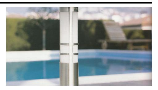
The **Border** bollard fitting is made from stainless steel and powder coated with a strong last lasting transparent varnish for additional protection from various weather conditions. The shade is made from borosilicate glass. Silicone gaskets are incorporated into the design to seal this 240V fitting from water. A fluorescent lamp source is used to increase energy efficiency when in operation.
