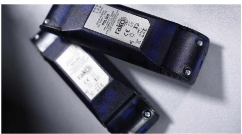
The RAKO Leading Edge Ceiling Mount Dimmer is designed to fit through the aperture of a standard low voltage down light fitting. The dimmer is connected in-line before the first light fitting, to enable dimming of up to 500W of leading edge dimmable loads. Suitable for use with inductive and resistive loads such as tungsten, low voltage halogen, cold cathode and other leading edge dimmable loads.
