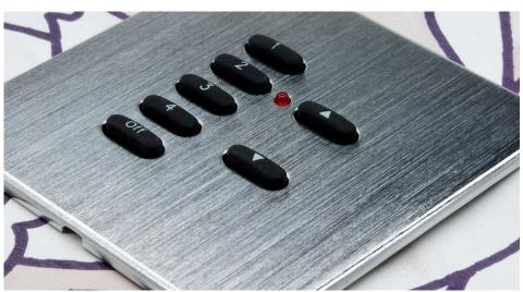
The **RAKO Wireless Wall Switch** is a 2 button wall mounted control panel providing on and off control functions. The on button recalls preset scene one. Lithium battery powered and using coded radio transmission eliminates the need for any data or power cabling, ensuring that the system can be installed with minimum fuss and disruption. Can be mounted anywhere, be it flush mounted to UK back-boxes or simply surface mounted to any flat surface using the patress provided.
