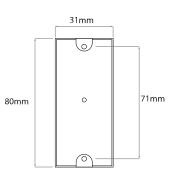
Single plate back box for use with single plate architrave switches requiring a shallow depth of 35mm. Cannot be used with our *Trimless Architrave Switches*.
