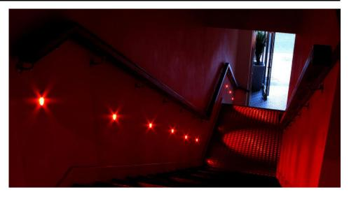
The **Quara Square** is a wall recessed spotlight used for indirect lighting. Its ideally used to highlight walkways such as corridors, paths and stairs. The Square has an IP rating of 65, enabling it to be used in a bathroom or outside.
