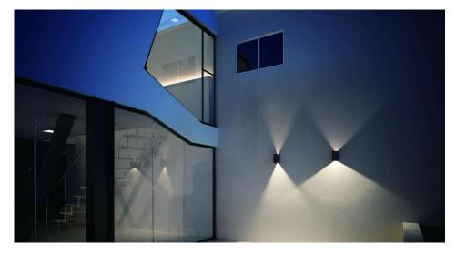
The **Adjustable Cross Beam 12W LED** can compose your desired light beams by adjusting the adjustable panels. The fitting has markings as a reference for the beam angles. With 4 x 3W Cree LED adjustable beam angle. Constructed of a die casting aluminium.
