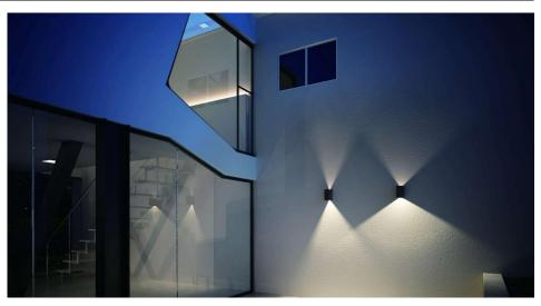
The Wide Adjustable Beam Wall 6W Up & Down LED can compose your desired light beams by adjusting the adjustable panels. With 2 x 3W Cree LED adjustable beam angle. Constructed of a die casting aluminium. Adjustable beam from 0-90°
