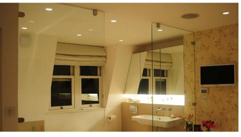
The **Trimless Double Round Downlight** is a fully adjustable downlight that is available in round or square, black or white. Using the different lampholders available you can select different light sources; Halogen, LED and Metal Halide. It is designed to be plastered into ceilings to give a **seamless** appearance. One of the advantages is that the downlight can be installed then plastered and painted.
