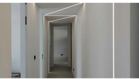
The **Kozma Extrusion Profile** is a slimmer profile for installation in drywalls, ceilings or grooves. The exposed aluminium wings can then be plastered over and painted to leave an elegant line of light. Creative compositions of narrow lines of light can be produced in the surfaces of walls and ceilings.
