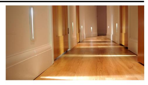
The **LED Blade RGB** colour changing low level recessed light that is used in walls. It has a waterproof rating of IP65, and a beam angle of 5°.
