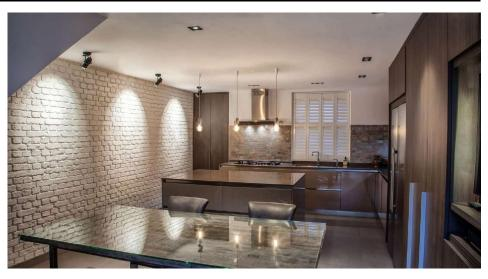
The PAR30 Theatre lights are 240V spotlights used to highlight certain focal points using different wattages, brightness, beam angles, filters and coloured gels.
