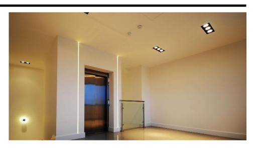
The **LED Grid Trimless Single AR70** is an adjustable downlighter with a **Reality AR70 LED 8W & Driver**.
