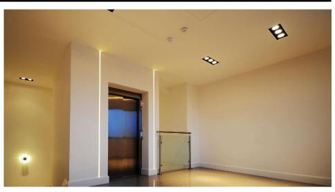
The **LED Grid Trimless Quadruple AR111** is an adjustable downlighter with four **13W AR111 LED Lamps & Drivers**.
