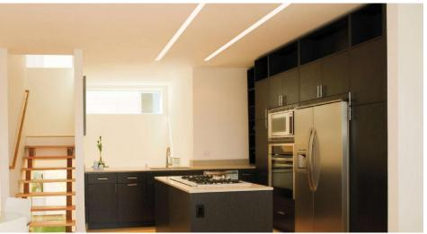
The **Micro Blade** extrusion is constructed from high strength plaster. It is used for indirect recessed lighting, ideal for walls and ceilings. LED strips recommended for use with this extrusion.
