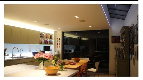
The **Trimless Downlight** is a fully adjustable downlight that is available in round or square, black or white. It is designed to be plastered into ceilings to give a **seamless** appearance. One of the advantages is that the downlight can be installed then plastered.
