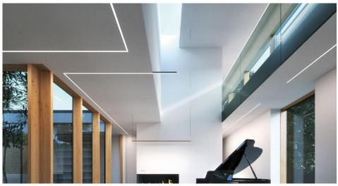
The **Larko Profile** is dedicated to be mounted into ceilings and drywall. Their height was designed the way that they can produce a single line of light with LEDs spaced 15mm apart and a frosted cover HS 22. The extrusion can accomodate two of the 10mm wide LED strips. Extrusion can be mounted to a surface with mounting springs.
