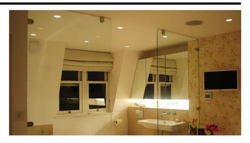
The **Trimless Downlight** is a fully adjustable downlight that is available in round or square, black or white. It is designed to be plastered into ceilings to give a **seamless** appearance. One of the advantages is that the downlight can be installed then plastered and painted.
