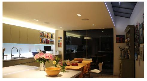
The **Trimless Downlight** is a fully adjustable downlight that is available in round or square, black or white. Using the different lampholders available you can select different light sources; Halogen, LED and Metal Halide. It is designed to be plastered into ceilings to give a **seamless** appearance. One of the advantages is that the downlight can be installed then plastered and painted.
