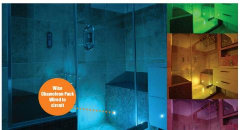
The Wise SyncroLED RGB Slave offers the same capability as your standard Chameleon yet with less wiring needed for it. The master receives the signal from the transmitter and then passes the signal on to the slave wirelessly without the need for cables between the master and slaves. Each pack only requires to be wired to a power supply
