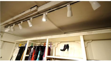
The **Long Nose Spotlight** is a three circuit track mounted spotlight used for general lighting. It has a longer body than standard GU10 spotlights, meaning that elongated bulbs such as LED retrofit lamps can be used without the light source protruding.
