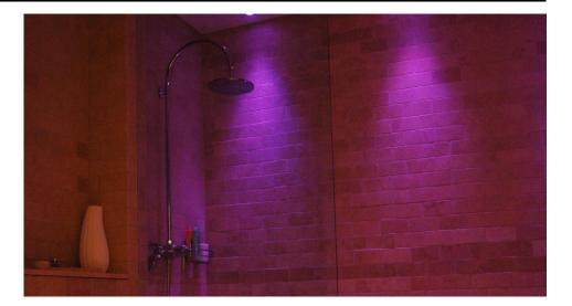
This retrofitted Happy LED Colour Changing Lamp and Remote is able to be fitted instead of a halogen dichroic lamp. This means that it is possible to fit it in most 50mm light fittings. The colour changing is operated by an IR remote. This means that the remote must be pointed at the lamp itself in order for colour changing to work.
