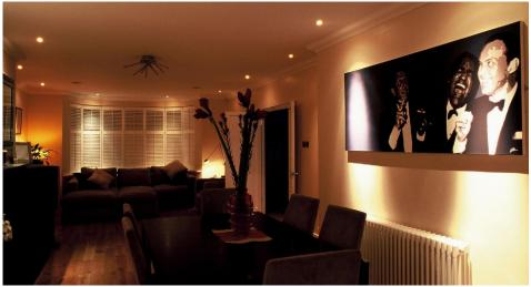
The **Rock 'n' Roll 35** is a fully adjustable 35mm downlight. The inner ring can tilt to a maximum of 35° for precise beam placement.
