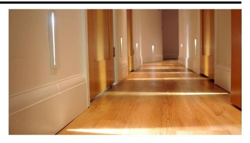
The **LED Blade** is a surface mounted fitting. It has a waterproof rating of IP54, and a beam angle of 5°.
