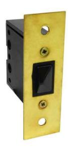
A **Door Switch** that enables you to turn a light on and off in a cupboard or room. When the door is closed on the switch the light would be turned off, as soon as the door is opened and the switch is released the light will turn on.
